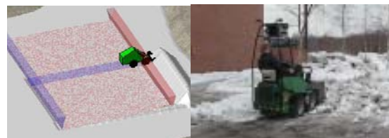
Figure 4. Bulldozing simulation with 3D graphical job planning tools (left). Outdoor test (right)
